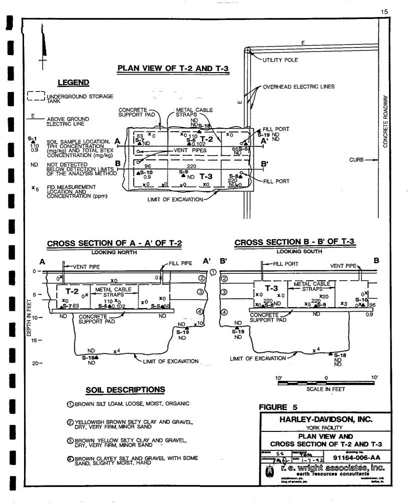
Backfilling of the T-2 excavation was completed on October 17, 1991. Soils removed during excavation of T-2 were used as backfill and compacted with the track-hoe bucket.
