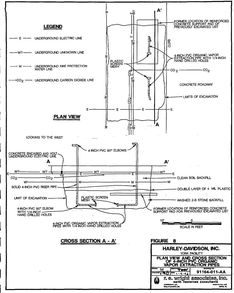
These 5-foot sections contain hand-drilled 1/4-inch holes on 1-foot centers, and had ends sealed with plastic mesh.
