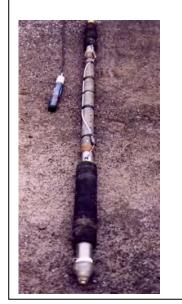
screen and adjacent to the conduit feature. At the ground surface, the equipment setup consists of a field computer, small injection pump and hose, reservoir with tracer, and a small generator. The packer assembly is positioned in place using a boom truck. A compressed air tank, regulator, and high pressure inflation line are required to inflate the packers.
