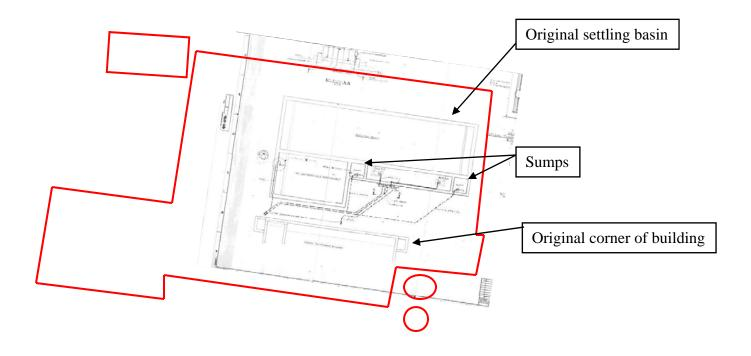
**Figure 2** – August 2, 1968 drawing with current WWTP outline shown in red. Note location of original lone settling basin, sumps, and northern corners of original WWTP Building.
