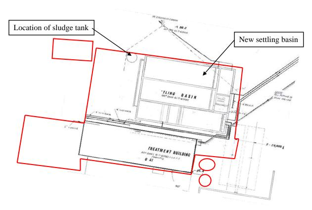
**Figure 3** – (1972?) drawing with outline of current WWTP shown in red. Note planned locations of settling basins; pipes from Bldgs 2 (east) & 4 (west); and location of sludge tank (W of North settling basin).
