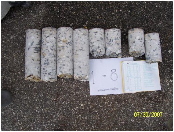
Photo 8 – View of concrete thickness at each of the eight boring locations.
