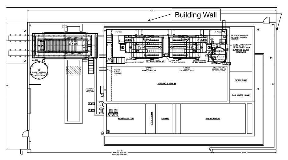
**Figure 4** – June 20, 2007 proposed (existing) layout [J. Mark Systems] showing Bldg 41 wastewater tank area only. Note proposed use of northern settling basin with a new lamella clarifier; new location of sludge filter press (indoors); and existing sludge pit (west of settling basins). Building walls and current roof over the WWTP basins was constructed circa 1980, according to other available construction drawings.
