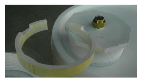
15. Place bag inside BFA, place ring on top of bag, and then screw 4" threaded male cap on top.16. After complete assembly, fill bucket with carbon to an inch over the top screened "W"
